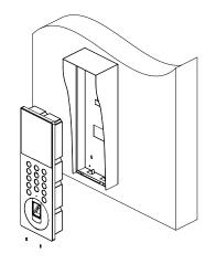
2. Connect the cables first, then align and push the locking tabs of the device into the rain cover. Use a hex wrench to tighten the two setscrews at the bottom.
