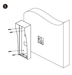
1. Align the mounting holes of the bracket with the holes on the wall. Insert the expansion tubes, and secure the rain cover to the wall with 4PCS SC-KA4X25 screws.
